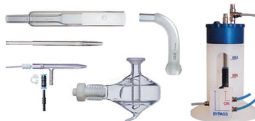
Figure 2. KT-1036 , High Solids Kit for iCAP 6000 Duo
