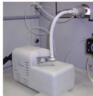
Figure 4. IsoMist Programmable Temperature Spray Chamber mounted on an Agilent 7500 ICP-MS
