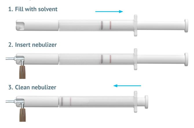
Particle build-up in a nebulizer capillary and tip causes sample flow to be constricted, thereby reducing nebulizer efficiency and performance. Now, blocked nebulizers can be safely and easily restored to optimum performance with the Eluo.
