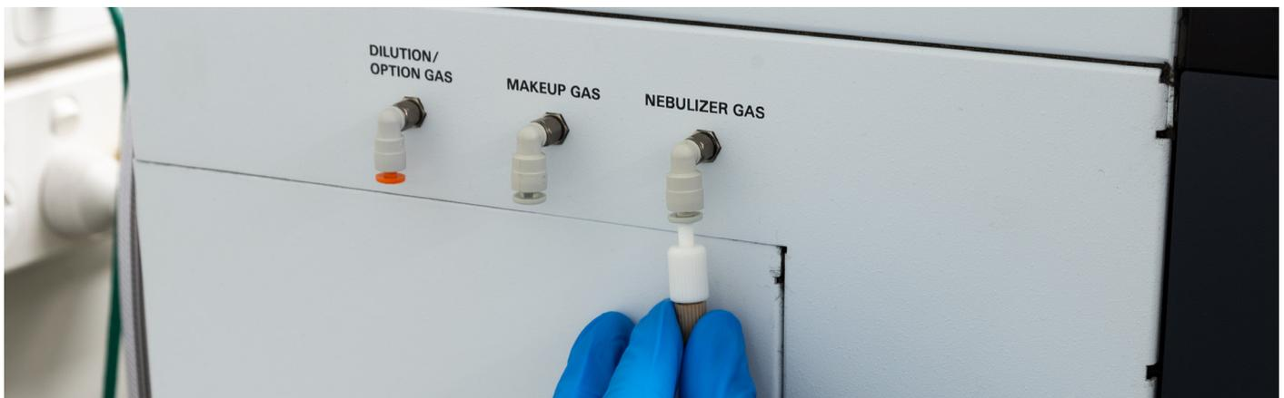
Figure 1 - Gas line 70-803-1105 shown as example.
