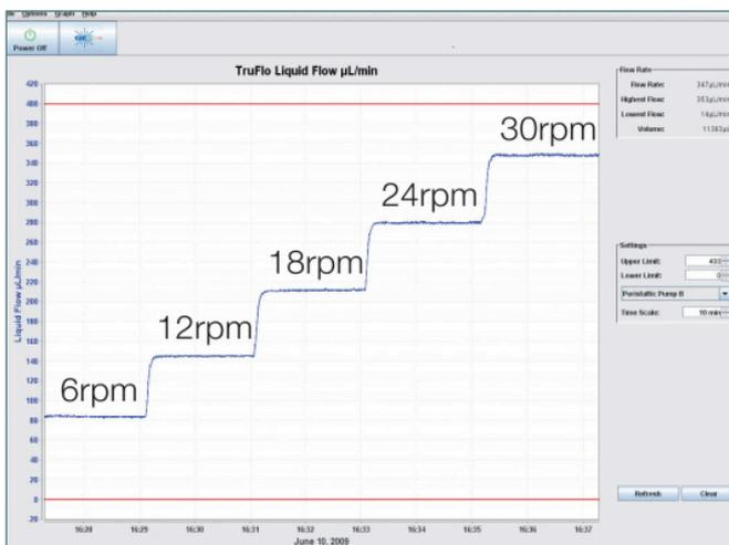
You always know the actual sample flow and you do not need to worry about converting pump revolutions to sample flow
