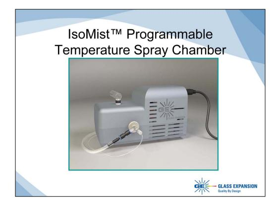
An IsoMist Programmable Temperature Spray Chamber (Glass Expansion) was used to vary the spray chamber temperature in the desired range. Shown above, the Peltier heat transfer component is housed to the right behind the company logo, while the nebulizer and spray chamber are to the left and a pumped drain line is configured below.
