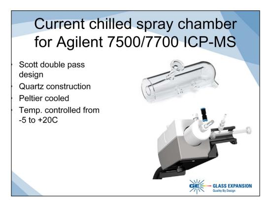
Agilent supplies a chilled Scott style double pass spray chamber with their ICP-MS instruments. The ChemStation instrument software controls the spray chamber temperature in the range of -5 to +20.
