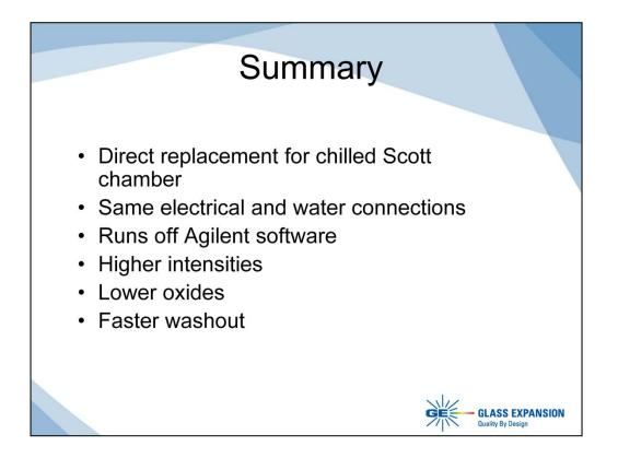
In summary, a chilled cyclonic spray chamber is now available for the Agilent 7500 and 7700 that is a plug-and-play replacement. It's advantages are higher intensities, lower oxides and faster washout.
