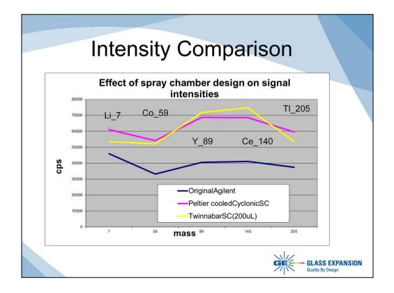
The intensity experiment showed large improvements when using either the Twister or Twinnabar. The Twinnabar experiment utilized half the sample uptake rate but also yielded a higher transport efficiency due to the smaller sample uptake rate.
