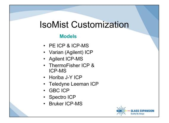
Configurations of the IsoMist are available which are customized for all of the models of ICP-OES and ICP-MS shown here. Furthermore, each one can be configured with a spray chamber made of borosilicate glass, quartz, or inert PFA.
