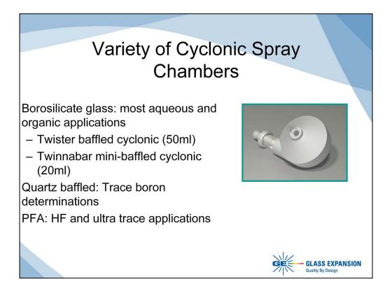
The glass and quartz chambers are encapsulated in a heat conductive resin. This serves two purposes; it facilitates heat transfer in and out of the chamber and it forms a tight seal with the heat transfer block eliminating any air which could otherwise result in condensation and freezing. The spray chamber is also available in HF resistant high-purity PFA.
