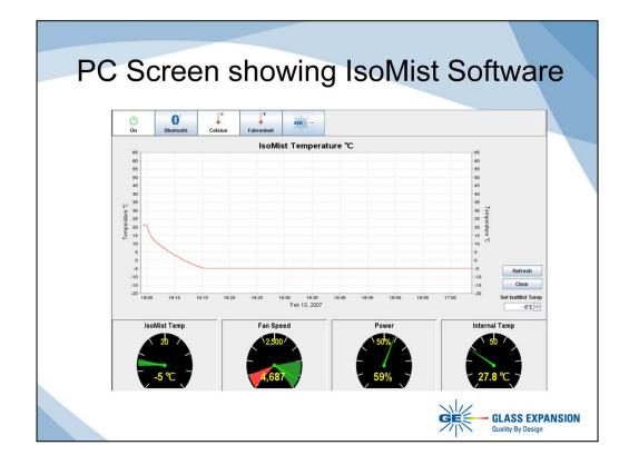
This is the one page proprietary application that controls the IsoMist. The temperature vs. time plots can be saved over the long term for regulatory compliance.
