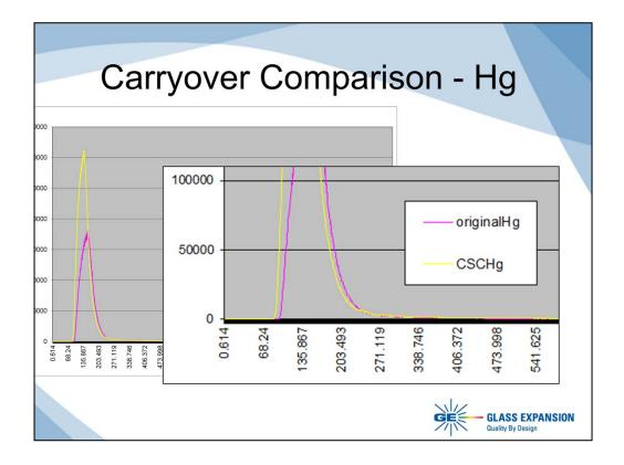
The graph on the left shows the full scale peaks and the difference in intensity is clear. The graph on the right shows a zoomed in view of the baseline. Despite the higher intensity, the Hg comes down to baseline at least as quickly as it does with the Scott style chamber.
