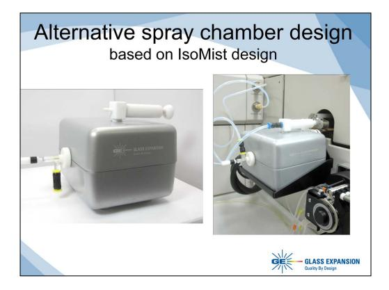
We designed a cyclonic spray chamber accessory that would be a plug-andplay replacement for the Agilent supplied chamber. It uses the same electrical and water connections (unlike the IsoMist, Agilent uses water cooling instead of air cooling) and runs off the same ChemStation software.
