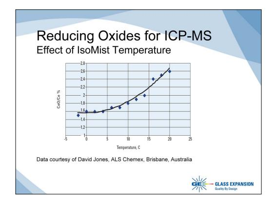
It is generally regarded that an oxide ratio of less than 2% is desirable to provide a more robust system. Even instruments which use collision/reaction cells to reduce oxide and other molecular isobaric interferences benefit from a reduced oxide ratio. In this experiment, it was found that using an IsoMist temperature of 2°C was optimum.
