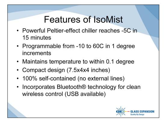
The features of the IsoMist are shown here. It should also be mentioned that the IsoMist "remembers" the last temperature at which it was set. Therefore, if you are using the same temperature daily, there is no need to connect it to a PC once it has been set.
