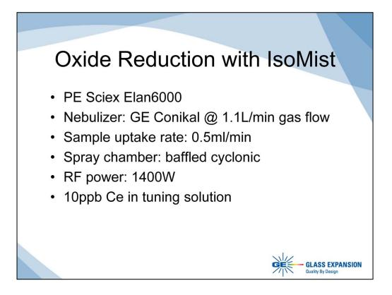
Using an Elan 6000 ICP-MS from PerkinElmer, David Jones from ALS Chemex in Brisbane, Australia, found that a nebulizer gas flow of 1.1L/min minimized oxide formation when the spray chamber was held at the appropriate temperature.
