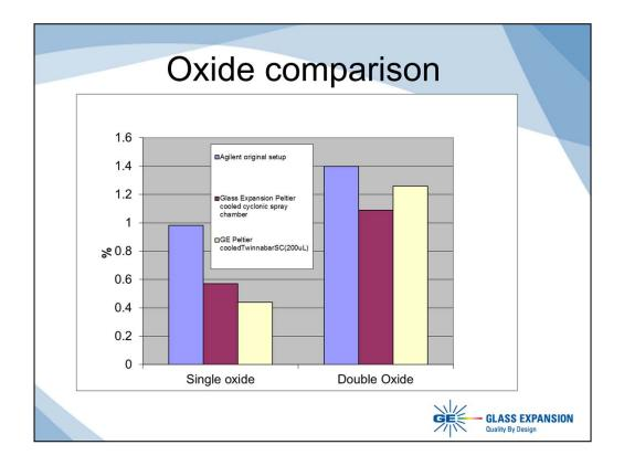
Comparing the oxide ratios, we found that the cyclonic spray chambers resulted in lower single charged and double charged oxide ratios than the Scott style design. For single charged species, the Twinnabar chamber was the lowest while the Twister had the lowest oxides for the double charged species.
