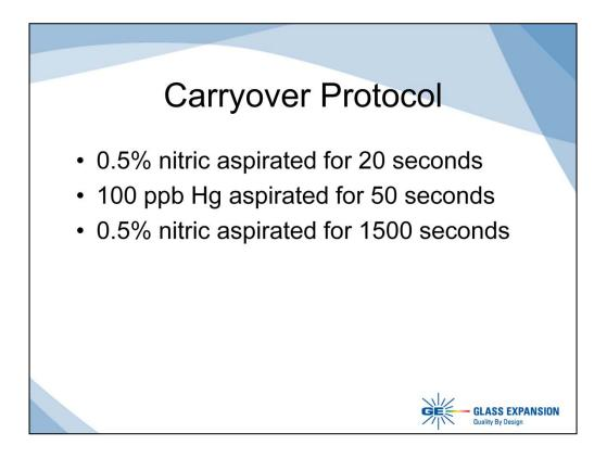
We also compared the carryover of the Scott style with the Twister. This was done by monitoring the Hg signal after a 50 second aspiration and monitoring it for 1500 seconds.
