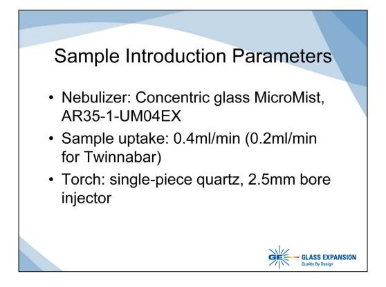
The standard Agilent MicroMist nebulizer was used at an uptake rate of 0.4ml/min. For the Twinnabar study, a lower uptake rate of 0.2ml/min was employed to emulate the normal conditions of a low volume spray chamber.
